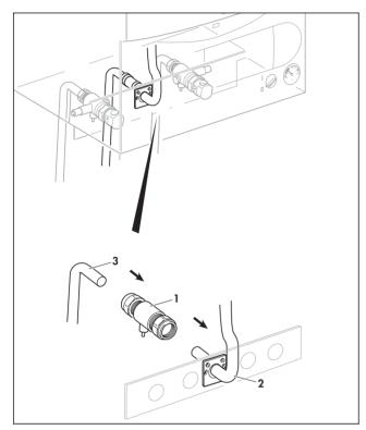
Fig. 5.9: Fitting the gas connection thermoCOMPACT
