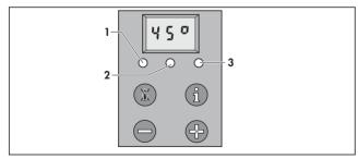
Fig. 8.3 Functional check turboMAX plus
