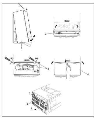
Fig. 5.21: Fit boiler casing
