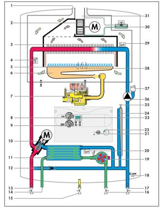
Fig. 3.3: Functional Diagram turboMAX plus
