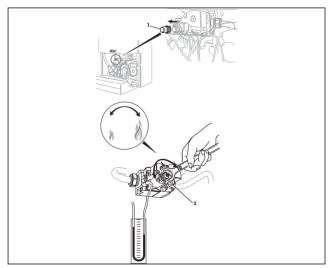
Fig. 7.4: Adjusting the ignition rate
