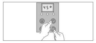
Record central heating operating pressure in the Benchmark Log Book along with the heat input (kW) and temperature difference between flow and return.
