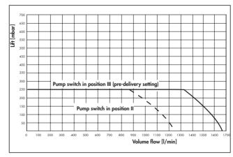
Fig. 4.6: Pump specifications 37 kW
