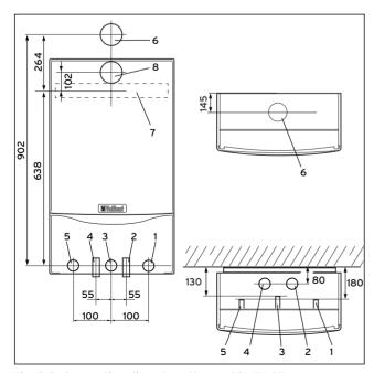
Fig. 3.2: Connection diameters thermoCOMPACT
