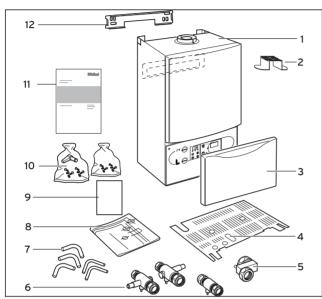
Fig. 1.1: Items supplied with unit (turboMAX plus)
