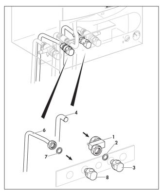
Fig. 5.7: Fitting the hot and cold water connections turboMAX plus
