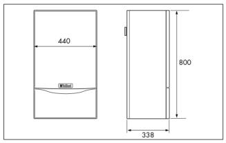
Fig. 5.1: Dimensions of boiler
