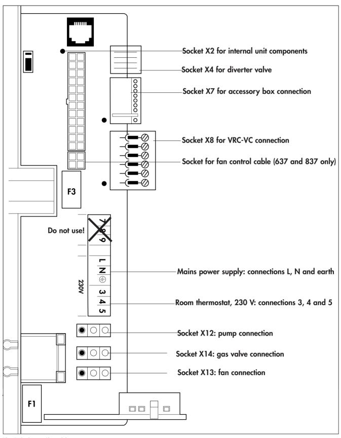
Fig. 5.13: Connection wiring
