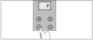
After setting, press and hold the "i" button for five seconds - or until the display stops flashing. The new setting value is now memorised. The new main burner pressure can now be checked. If the new output is not correct repeat steps 3 to 5.
