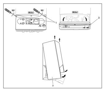
Fig. 5.5: Remove of boiler casing
