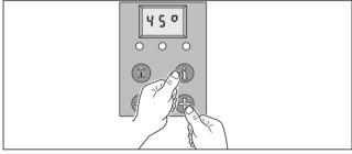
Keep the "+" button pressed until "d.0" is displayed. (The display runs from "d.0" to "d.99" before restarting again at "d.0".)
