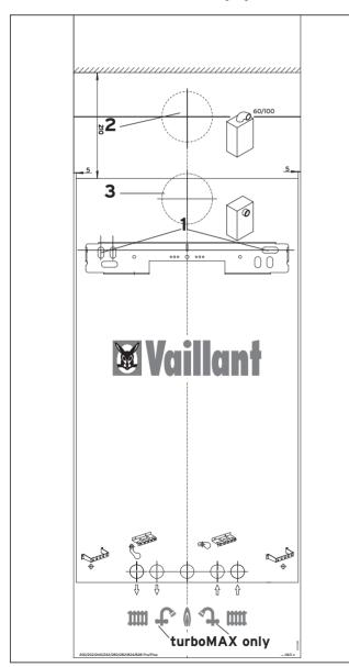
Fig. 5.3: Using Boiler template
