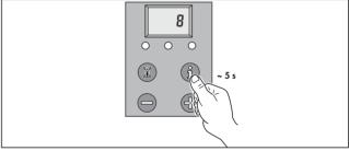
• To return to normal mode, press the "i" and "+" buttons simultaneously.
