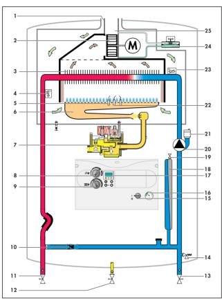
Fig. 3.4: Functional Diagram thermoCOMPACT
