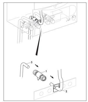
Fig. 5.6: Fitting the gas connection turboMAX plus
