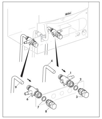
Fig. 5.10: Central heating flow and return pipework thermoCOMPACT
