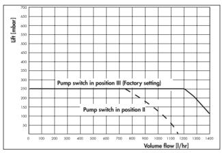
Fig. 4.6: Pump specifications 12-28 kW
