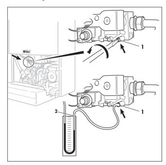
Fig. 7.1: Gas inlet working pressure
