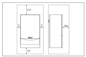
Fig. 5.2: Free space required for installation
