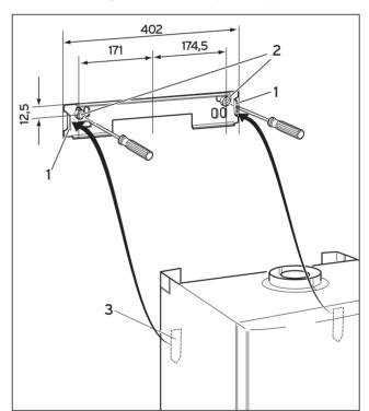
Fig. 5.4: Free space required for installation
