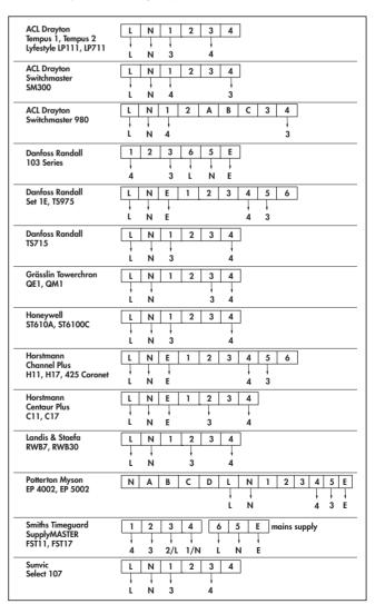
Fig. 5.15 Connection details for time switch
