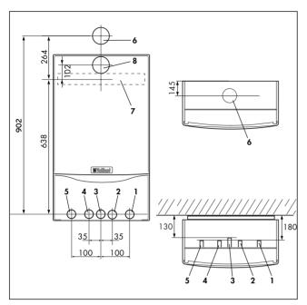
Fig. 3.1: Connection diameters turboMAX plus
