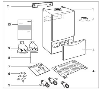
Fig. 1.2: Items supplied with unit (thermoCOMPACT)
