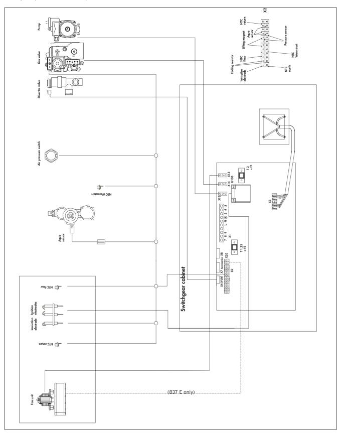
Fig. 11.3: Wiring diagram VUW
