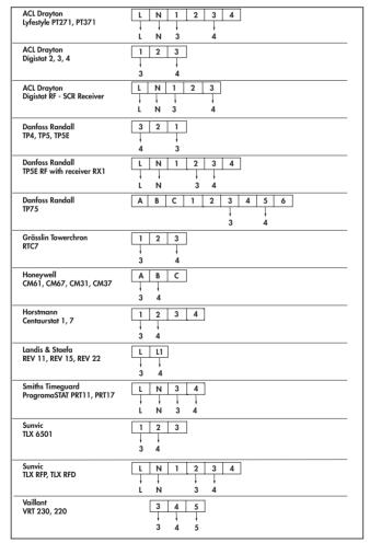
Fig. 5.14 Connection details for programmable thermostats
