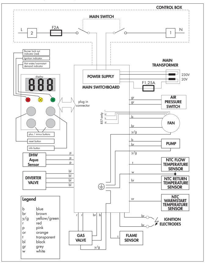
Fig. 11.1: Functional Flow diagram VUW
