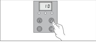
Use the "+" or "-" buttons to increase or decrease the value. Observe the U-gauge as the button is pushed and stop pushing when the required main burner pressure has been achieved.
