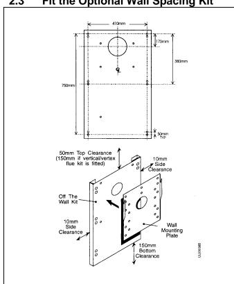
The wall spacing kit allows the boiler to be spaced 40 mm from the wall, providing sufficient room for all pipework to be run behind the boiler.
