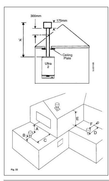
Minimum Flue length (dimension A) 1.2m
