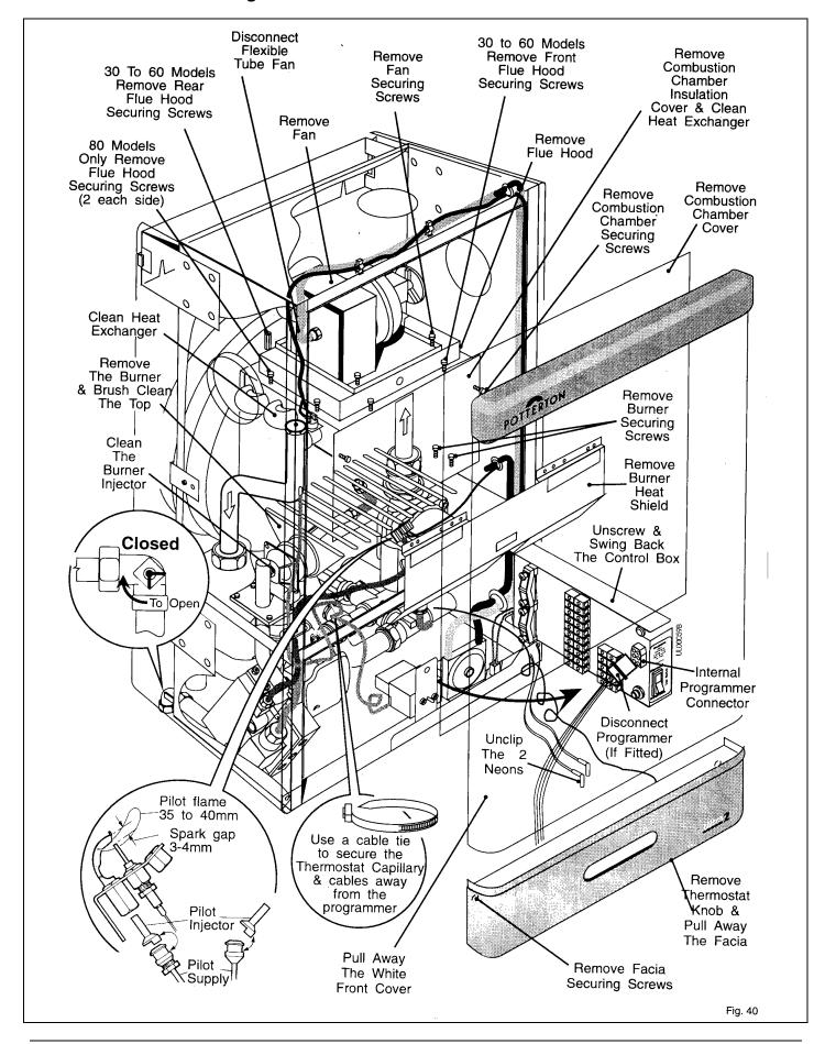
WARNING: Before commencing work open, the control panel cover (hinges down) and turn the thermostat knob to O (Off).
