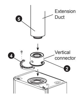
6. If the last extension duct requires cutting, measure 'X', the distance (outer ducts), between the duct and the terminal and add 100 mm to this dimension. This gives the length of the last extension duct.
