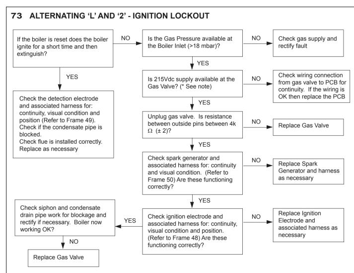
\* Note: due to the wave form of the rectified voltage, the reading will vary depending on the type of meter used to measure the value. In general terms a reading greater than 150V indicates that the correct voltage is supplied to the gas valve.
