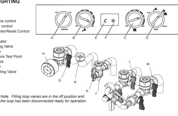
1. Check that the system has been filled and that the boiler is not IMPORTANT airlocked. Ensure the automatic air vent cap is open. Note.
